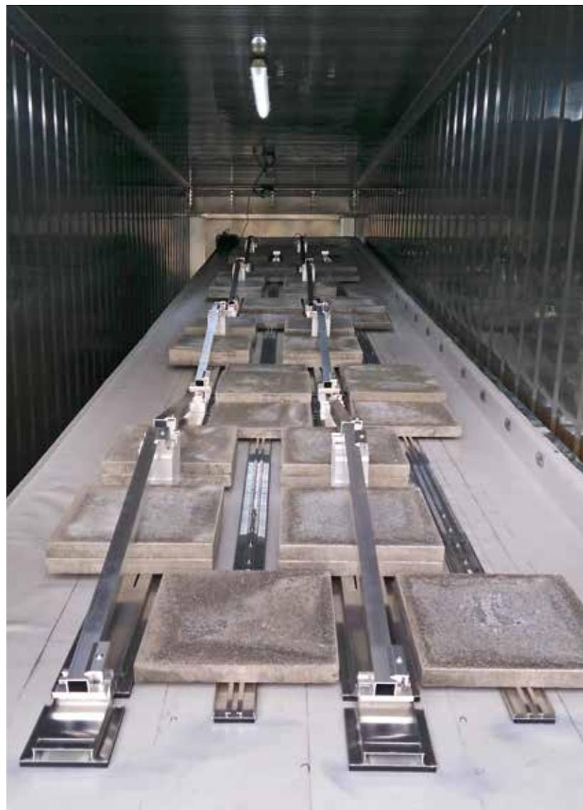
Layout of the PMT climate container. The left rail is connected to the test roof via a force measurement device. The right rail is not connected. The test is designed to show whether the right rail is moving and how much force is required on the left rail to suppress the movement.
